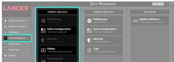
4. Tap *Valve Configuration* under the Import USB Data pane to import valve brand mapping data.
