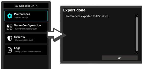
4. Tap the *Valve Configuration* button under the Export USB Data pane to export valve brand mapping data.
