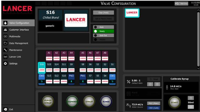
3. Adjust the desired dispense amount to 50 ml using the +/- buttons in the Calibrate Syrup pane.
