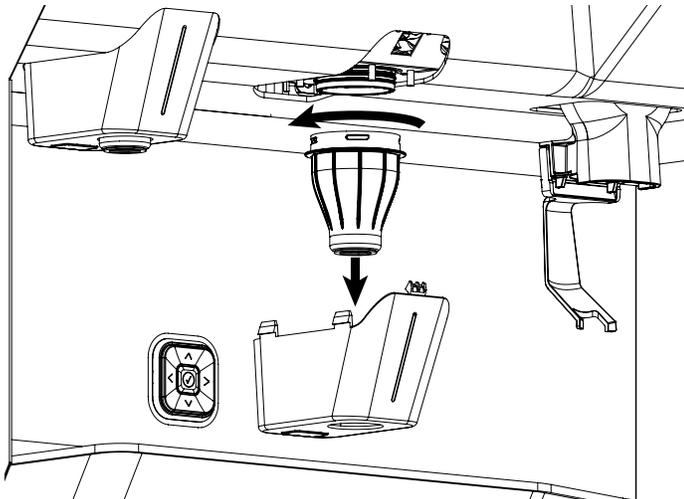
3. Insert syrup separator into outer nozzle.
