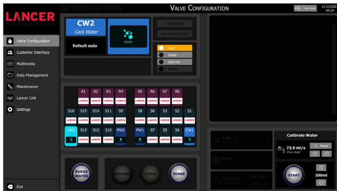
3. Adjust the water flow rate to 73.9 ml/s using the +/- buttons in the Calibrate Water pane (roughly equates to 2.5 fl oz/s, which is normal for a 3.0 fl oz/s finished drink).
