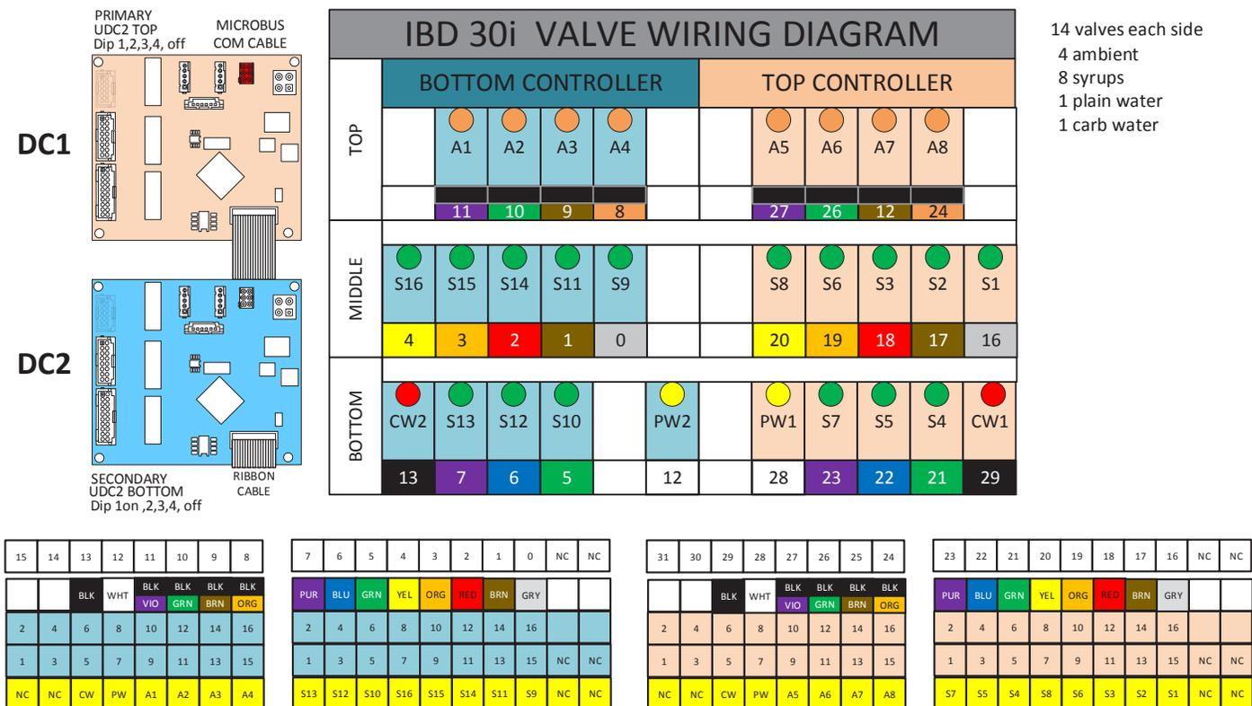
52-4167 left side valve from bottom secondary UDC2 (Short Harness)
