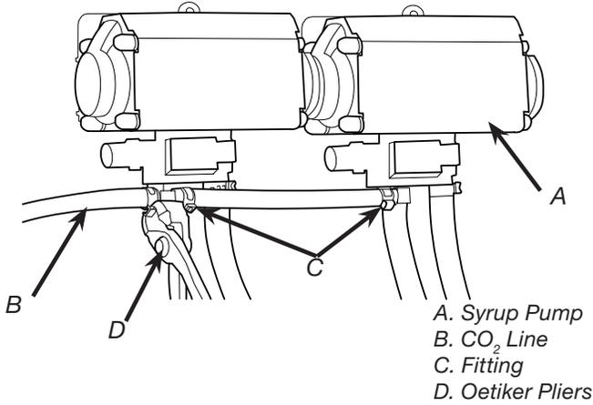
3. Using tubing cutters, cut the CO<sub>2</sub> supply line to the syrup pumps and install tee fitting. Then, route the appropriate tubing from the tee fitting to the syrup pumps and to the unit.
