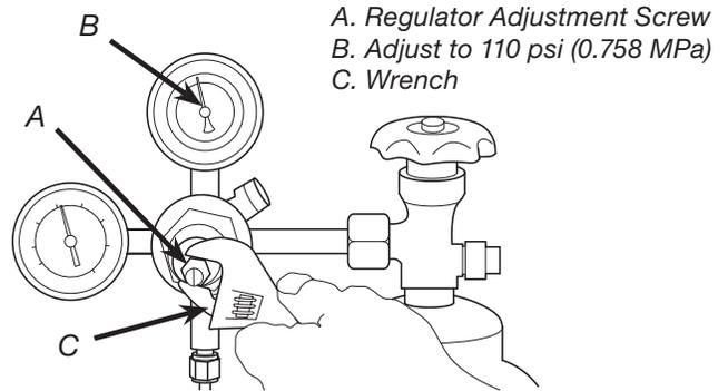
7. Adjust both of the low pressure regulators on the regulator manifold to 75 psi (0.517 MPa) then tighten locknut with wrench.
