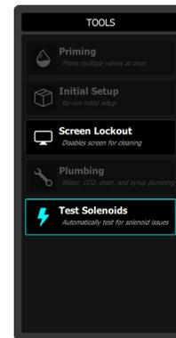
6. Tap *Start Solenoid Test* to begin testing of all valves.
