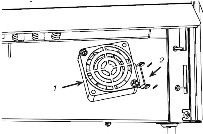
2. Connect the unit's red and black power harness to fan connector.
