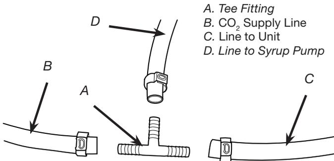
4. Connect tubing from dispenser syrup inlet to the syrup pump outlet fitting. Repeat for each syrup line/pump.
