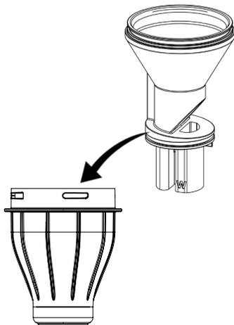
4. Reattach outer nozzle by pushing up and twisting clockwise until snug.
