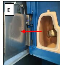
**2** Locate the cup sensors underneath the front door. Use a damp cloth and wipe them down.
